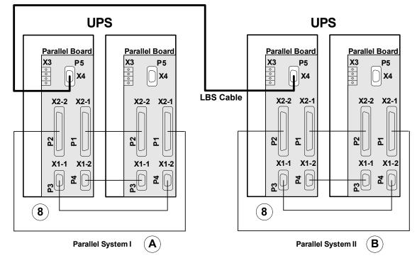
Figure 13 Load Bus Synchronization cable connection with multi-module systems
